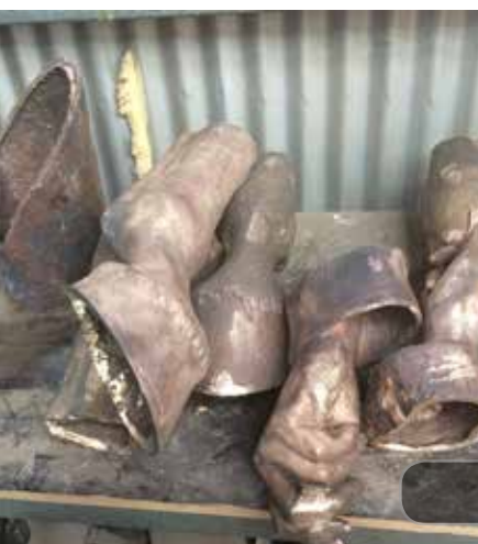
Part of bronze casting of Horseman no 2 before assembly
